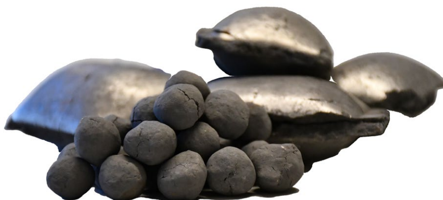
Manufacturing of sponge iron through direct reduction using hydrogen. Photo: Åsa Bäcklin. Source: HYBRIT
